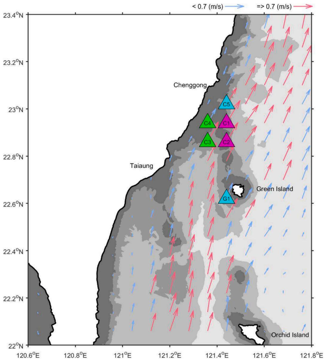
**Fig. 8.** Typical drifter speeds as well as the 6 suitable sites located east of Chenggong (C1–C5 sites) and southwest of Green Island (G1 site). The contours represent the isobaths (–500 m, –1000 m, and –2000 m). Red (blue) arrows indicate a current speed greater (less) than 0.7 m/s. (For interpretation of the references to colour in this figure legend, the reader is referred to the web version of this article.)
