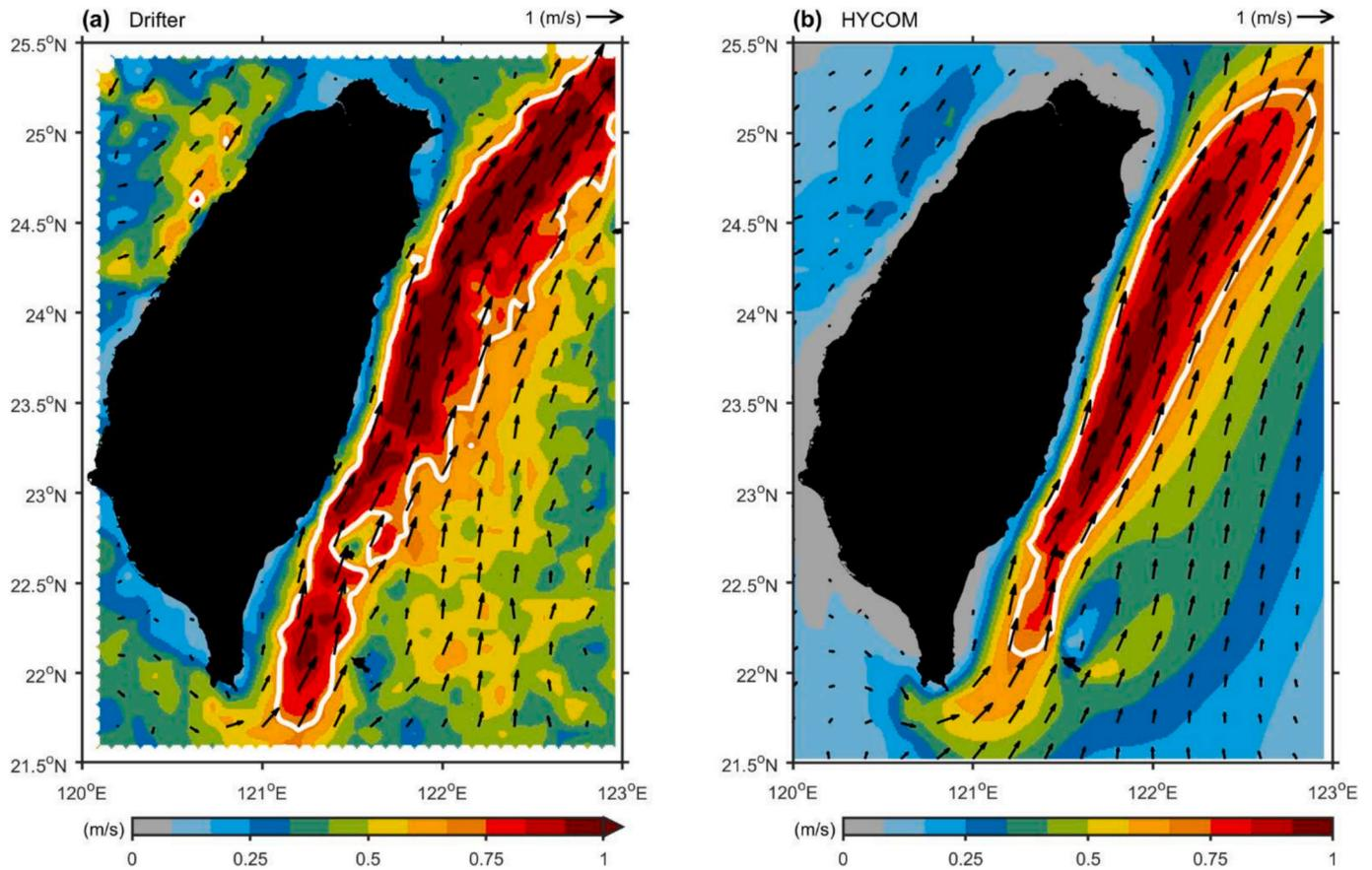
Fig. 4. Temporally averaged current speeds and vectors from (a) drifter data and (b) the HYCOM+NCODA 1/12° reanalysis data at 15 m depth.
