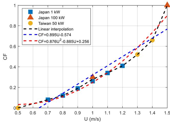
**Fig. 10.** Relationship between towing (current) speeds and the capacity factor (CF) for ocean current turbines.
