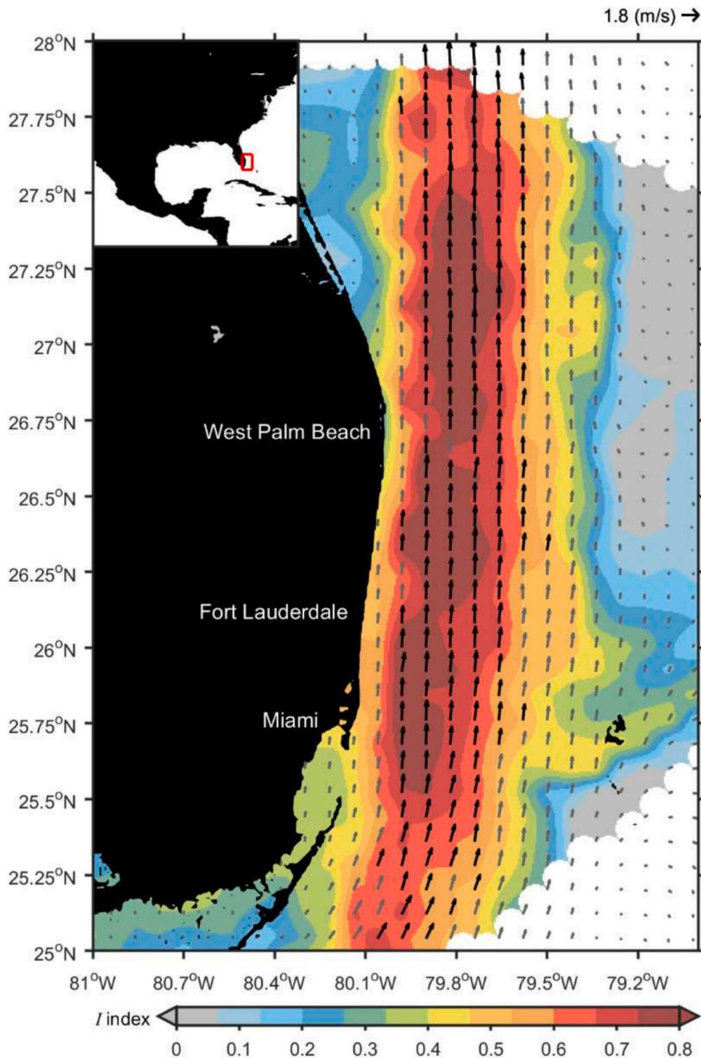
**Fig. 16.** Distribution of the feasibility index ( $I$ ) in the Gulf Stream region. Averaged drifter velocities (arrows) in  $1/12^\circ \times 1/12^\circ$  bins. Speeds higher and lower than 1.2 m/s are shown in black and gray, respectively.
