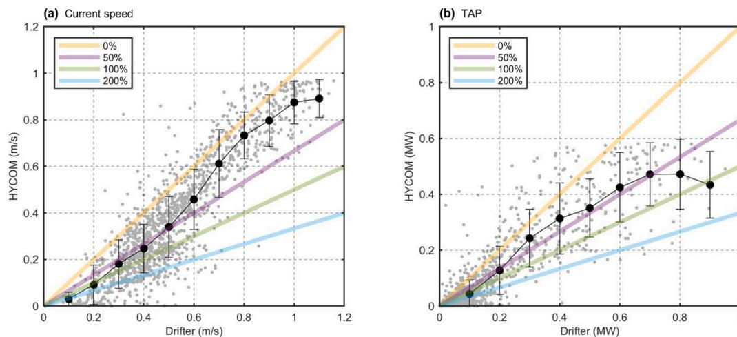
**Fig. 15.** (a) Current speeds based on GDP drifter data and HYCOM-NCODA reanalysis data (GLBu0.08). (b) TAP for a 2 MW current turbine based on GDP drifter data and HYCOM-NCODA model data. Oblique lines represent the percentage increase in drifter speed and TAP. Black dots represent the mean percentage increase in drifter speed and TAP with the error bars showing one standard deviation.
